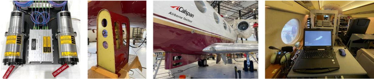
Fig. 7 LoRA Engineering Unit, Sensor Fairing, Testbed Aircraft, and In-Cabin Engineering Station
