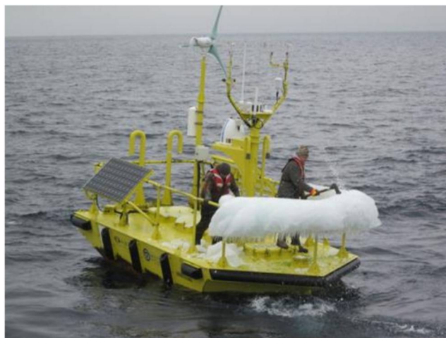
Figure 14 – WindSentinel with excess ice build-up on bow railing being removed by crew.
