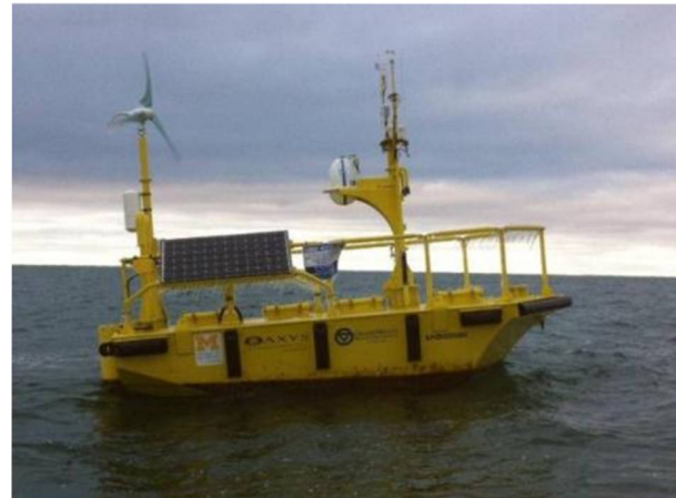
Figure 1 – WindSentinel Floating MET Facility
