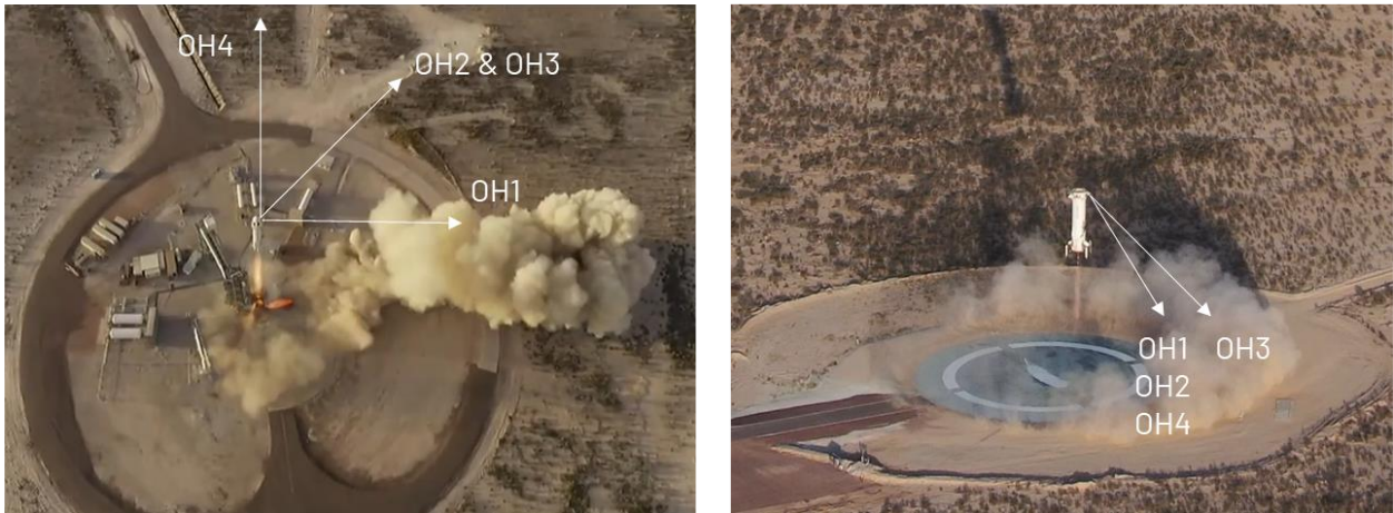
Figure 12: Dust plumes for Flight 1 at liftoff (left) and landing (right) confirming dust affecting recorded data.
